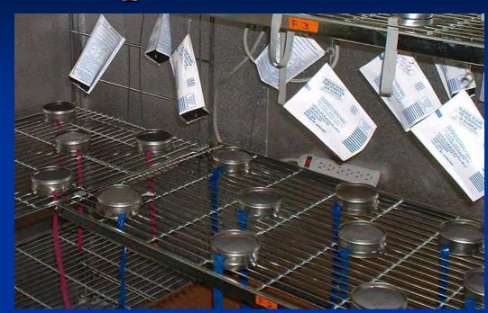
Canisters, Bags, Trays: analyzed by gamma spectroscopy
