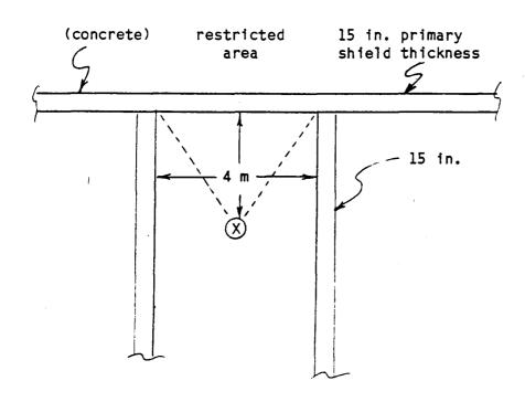
Beam is incident only on primary shield wall.
